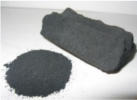
Activated Carbon is a piece of charcoal activated by oxygen. source: http://commons.wikimedia.org/wiki/File:Activated_Carbon.jpg
